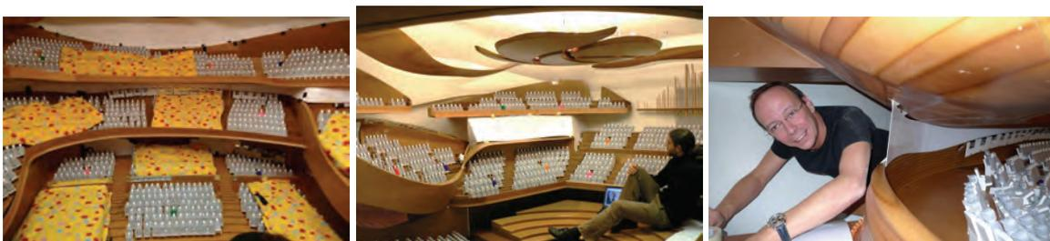
Figure 1. Model interior. Additional absorption and installation of coupling surface closures.
