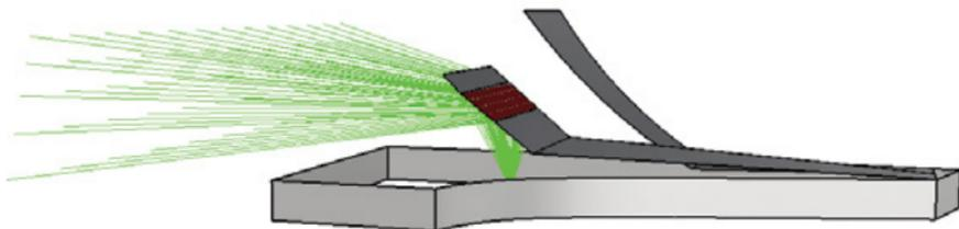
original lid, with the split lid (that is, the flexible backward-projecting lid), with the final version of the box, and with the final version of the horn. The results, summarized in figure 6, reveal the true acoustic effect of the different hearing machines (expressed in decibels) for different frequency bands (expressed in hertz). The first case—without lid—was chosen as our reference, corresponding to 0 dB, onto which the other four cases have been mapped.
