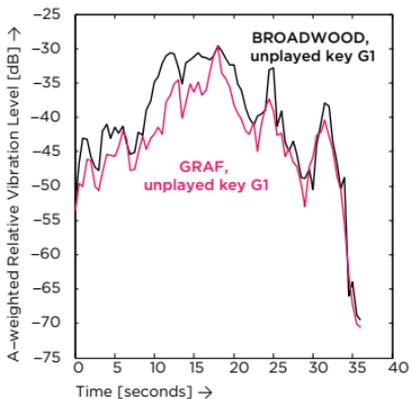
**FIGURE 7** Vibration level measurements on Broadwood versus Graf, with accelerometer on an unplayed key. Opus 109, third movement, fourth variation, mm. 105<sup>2</sup>-112.
