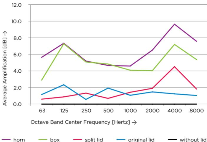
**FIGURE 6** Amplification effects of the various hearing machines and lid settings.
