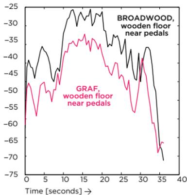
**FIGURE 8** Vibration level measurements on Broadwood versus Graf, with accelerometer on the floor. Opus 109, third movement, fourth variation, mm. 105<sup>2</sup>-112.
