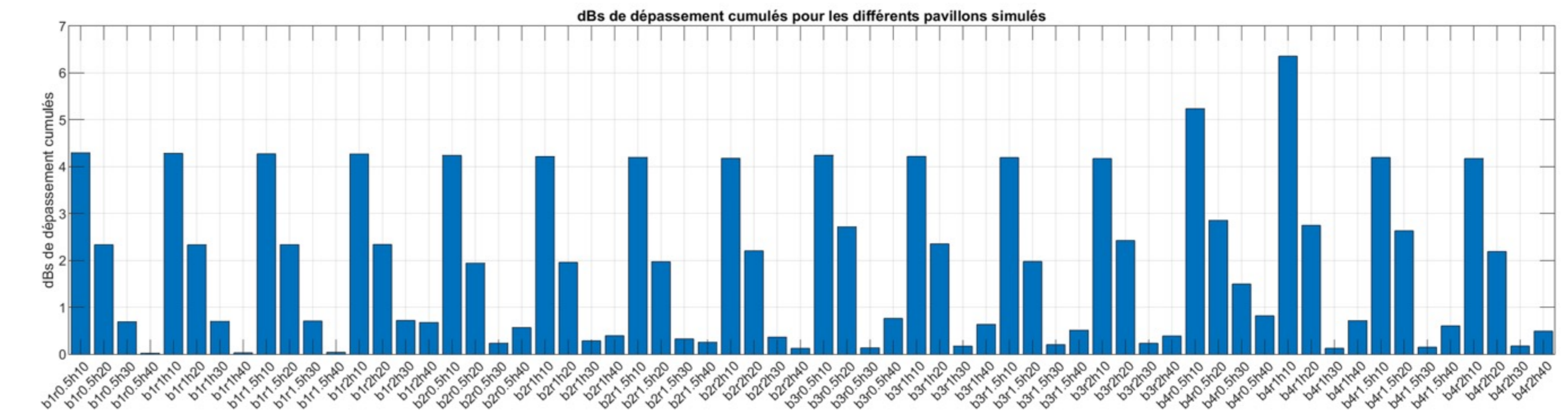
Comparison of the cumulative deviation of directivity for all 64 simulated models compared to the standard ISO 3382-1
