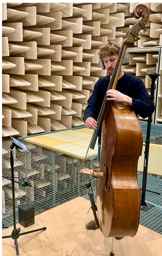
Fig. 3. Musician in the experimental set-up: Extra-aural headphones, head tracker, microphone, tablet, talk-back speaker, wooden floor plate; rendering computer and audio interface located outside the room.
