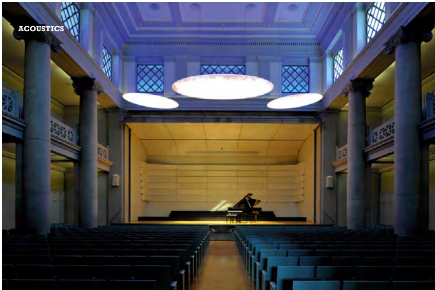
Above: Stadthaus Winterthur in Switzerland with the new stage shell. The ellipsoidal lights provide reflections back to the musicians and to audience in the stalls. Photo: Karl Fülischer for Architekturbüro Johann Frei
